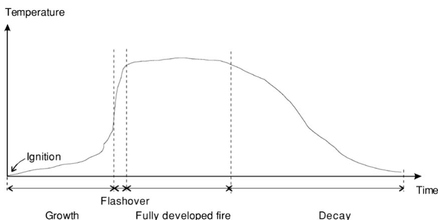
**Figure 1. Idealised description of the temperature development with time in a compartment fire**
