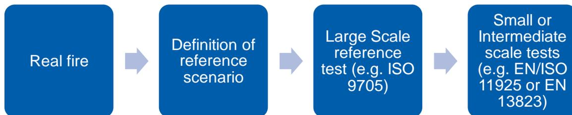
**Figure 1 Schematic describing the CPD/CPR classification system (based on Notified Bodies Position Paper<sup>5</sup>)**
